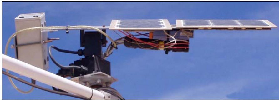
Figure 3.4: SCTU mobile platform pointing to the sun
