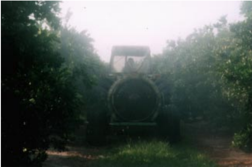
Figure 5: a manually-driven tractor pulls an airblast sprayer to apply pesticides to citrus trees.
