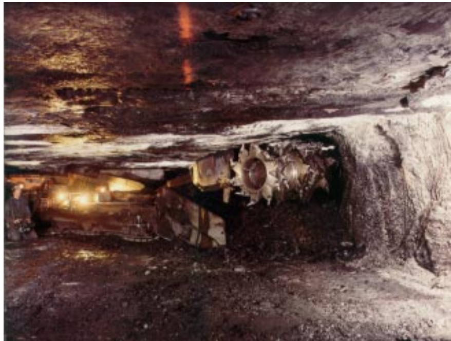
Figure 3: A continuous mining machine extracts coal from a seam. The cutter head spins to shear the coal from the face. The machine collects the coal and deposits it in a shuttle car or mobile conveyor that follows (courtesy of Joy Mining Machinery).
