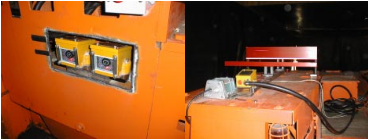
Figure 4: Left photo: SDM stereo cameras mounted on the side of CMU's continuous miner. Right photo: GHM planar targets with imaging camera (small box with cable) mounted on top of the continuous miner.
