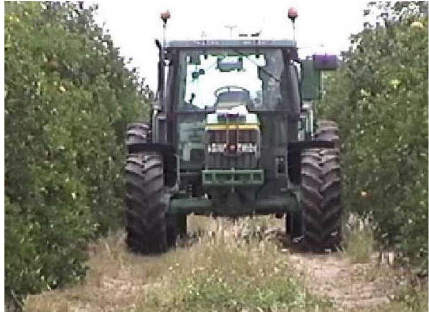
Figure 6: CMU's autonomous tractor sprays water in a grove in Florida. The tractor is guided by GPS with cameras for obstacle detection.
