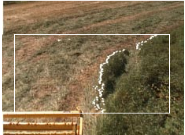
Figure 4: Sample output from the crop line tracker.
