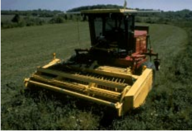
Figure 1: The Demeter automated harvester.
