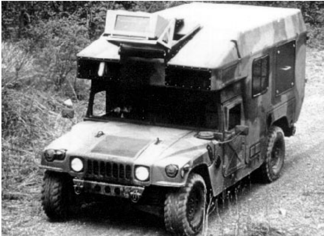
Figure 1: NAVLAB II Robot Testbed
