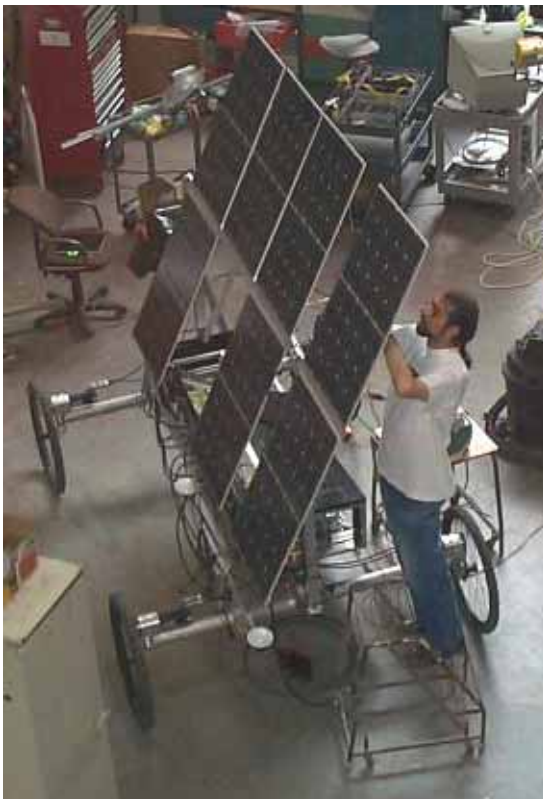
Figure 4 Hyperion solar-panel assembly
