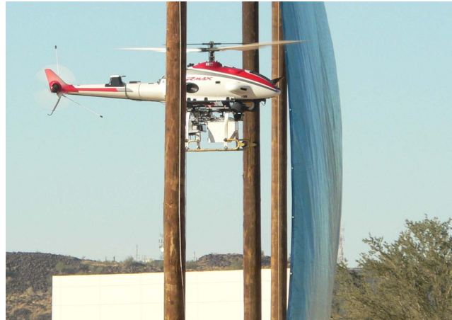
Fig. 1. The helicopter platform we used to test collision avoidance is flying autonomously in between two poles 10 m apart. The rotor span of this helicopter is 3.4m
