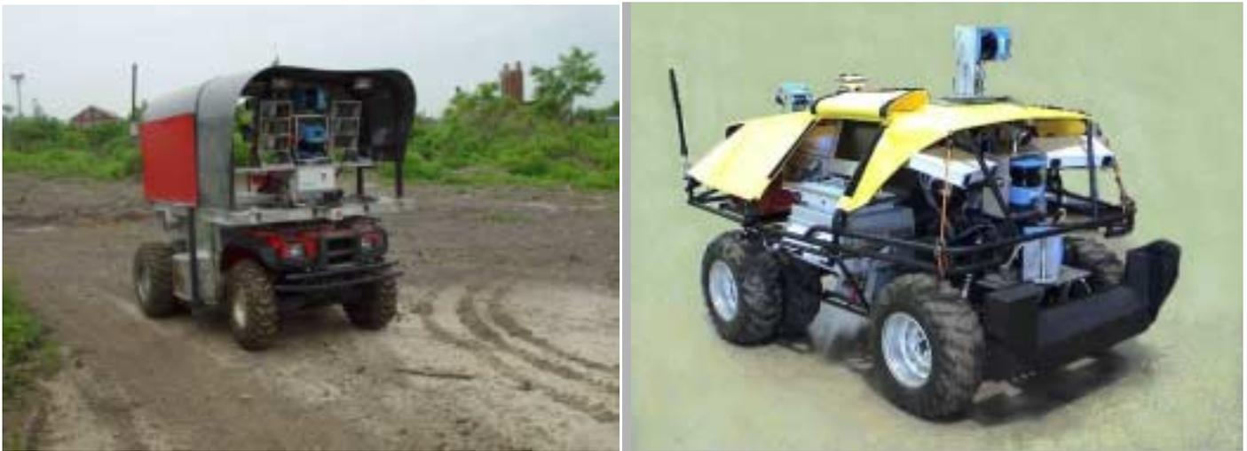
Figure 1. First (left) and second (right) generation UGV test vehicles based on the Honda Rubicon ATV platform.
