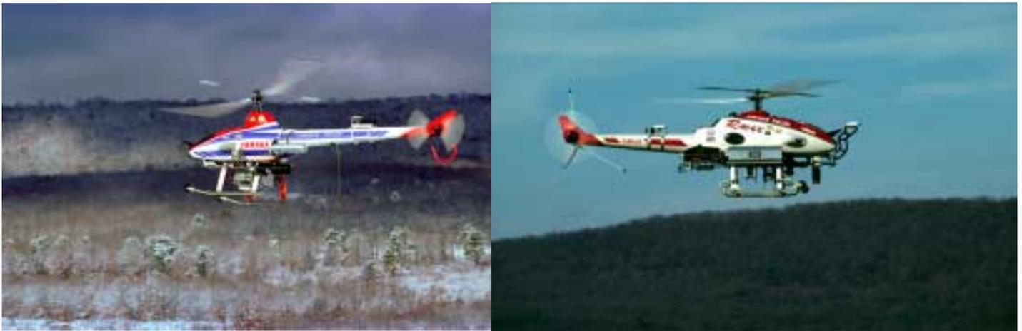
**Figure 3.** The Yamaha R50 autonomous helicopter (left) and the Yamaha RMAX autonomous helicopter (right).
