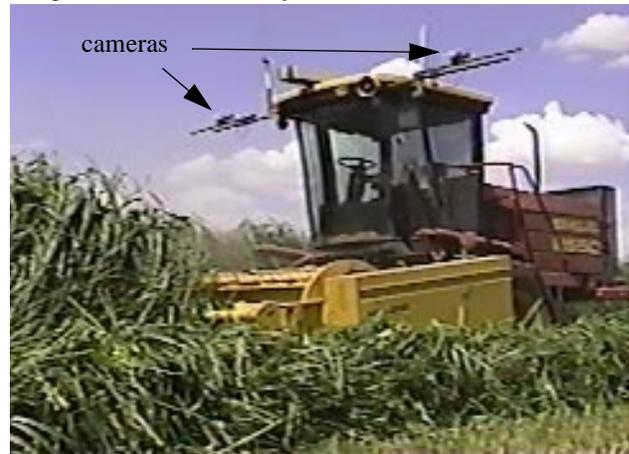
Figure 1: The Demeter automated harvester.
